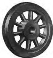
Fig. 4567. Steel Tired Wheel with Cast Iron Spoke Center. Tire Shrunken On.
